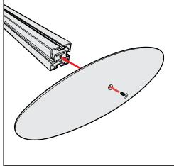
Base Plate & Extrusion Connection
